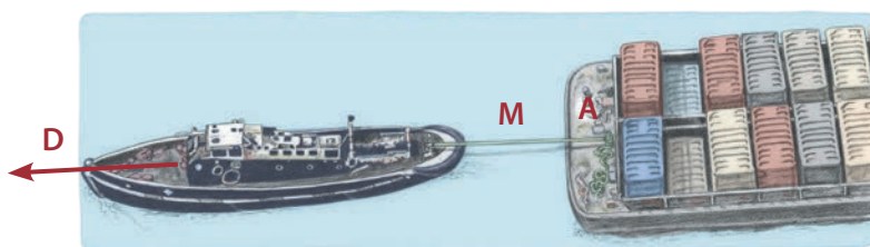
12.33 A tugboat applies direction, magnitude, and a point of application when pulling its load.
